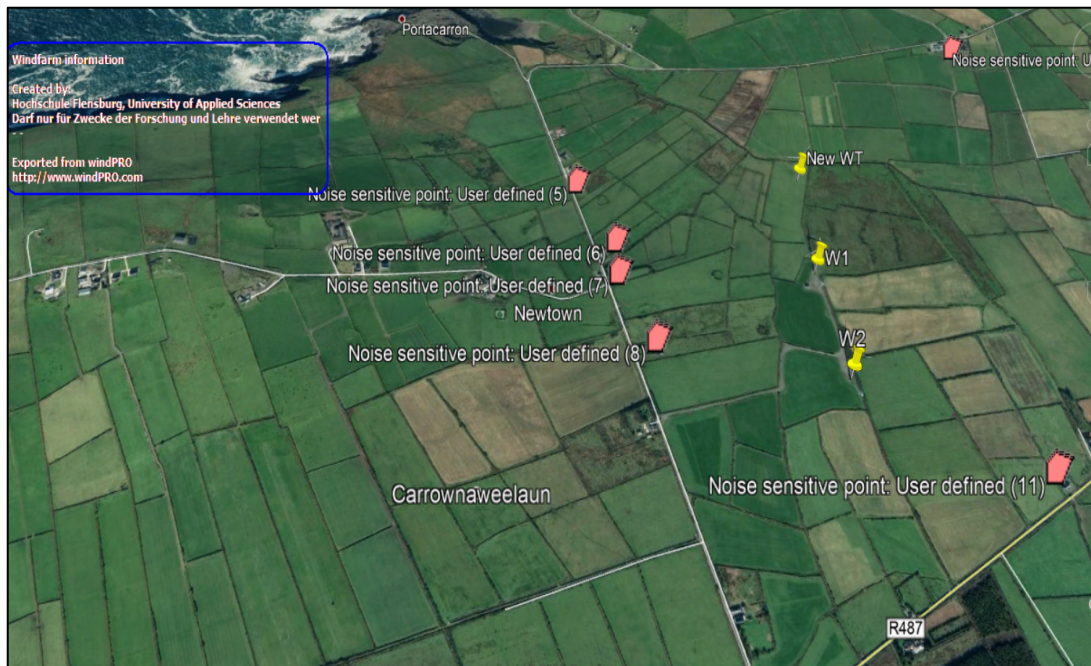
Figure 10-7: Noise Sensitive Areas as shown in Google Map (Source: Author's calculation using WindPro, Data Source: (EMD))
