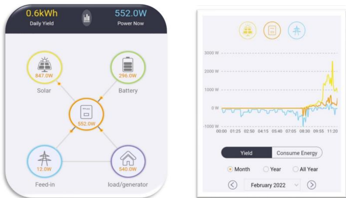
Figure 4.18: Mobile app for solar PV system performance monitoring Source:(Leonard, 2022a)
