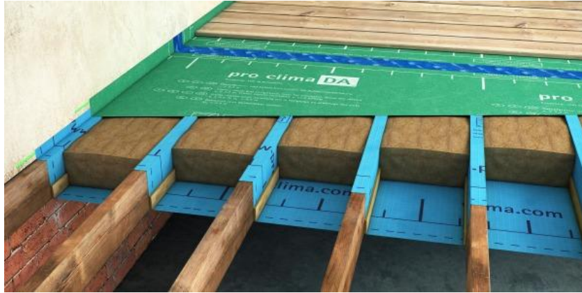
Figure 4.5 Wooden floor insulation Source: (Dave Judd, 2021)
