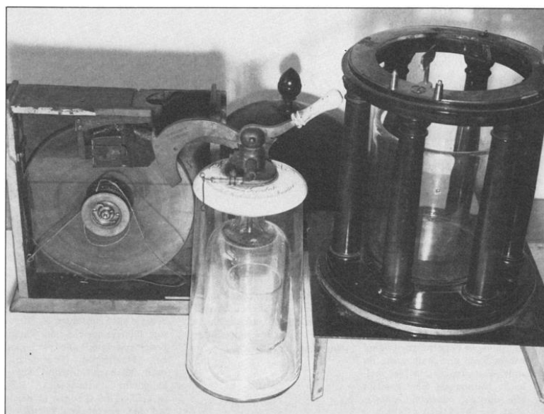
Fig. 11 Another Zündmaschine manufactured by Gerzabeck where it is possible to see how the device appears once it is opened and disassembled (Rehfus [n.d.]).
