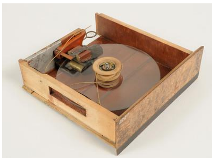
Fig. 10 Photo of how the electric machine appears once the wood base is opened. This particular example is from another Zündmaschine manufactured by Gerzabeck in 1830 and kept in the Deutsches Museum depot. © Deutsches Museum. Available at: http://www.deutsches-museum.de/blog/blog-post/2015/06/18/tischfeuerzeug-von-johann-gerzabeck/ (23/08/2020)
