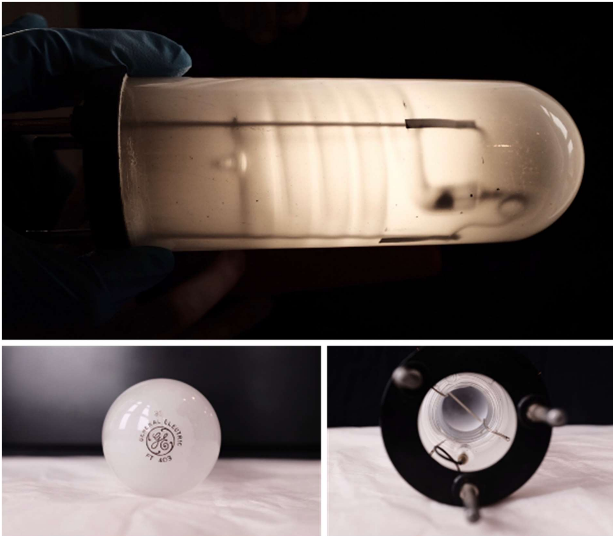
Figure 3, top: The artifact shown in backlighting. Bottom: The inscriptions of the dome of the artifact (left) and the bottom with a glance inside the cylinder (right), the different type of metal pins for stabilization and contact are clearly visible. Source: Deutsches Museum Munich © Nana Citron.
